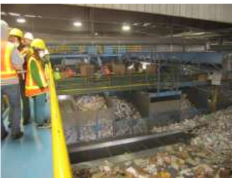
Recyclables that have been sorted at the Material Recovery Facility (MRF)
