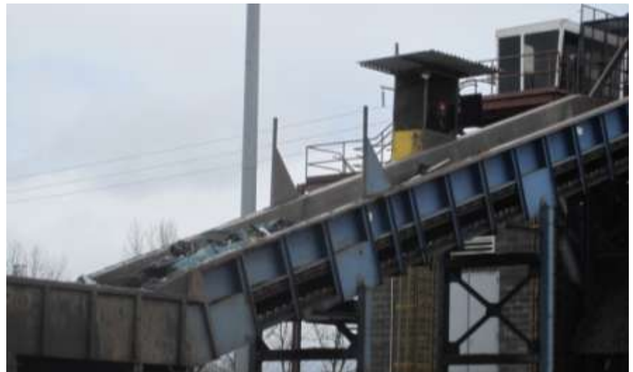
This conveyor belt carries scrap metal to the “jaws” to be shredded. Clad with 6 steel teeth that are changed daily, the tumbler can shred a full sized automobile. You can just see the top of a crushed sedan in the bottom left of this photo.
